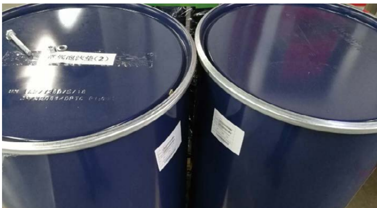
Risk of fingers pinched at the point of two barrels' contact
