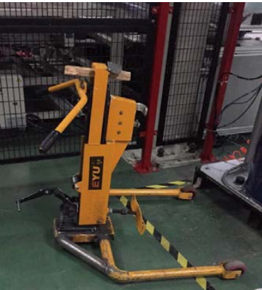
Use of hydraulic barrel clamp-forkliftvehicle
