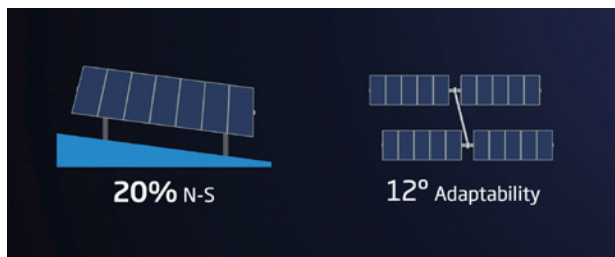
Image 24: Two slewing drives allow 12° terrain adaptability and 20% slope N-S
