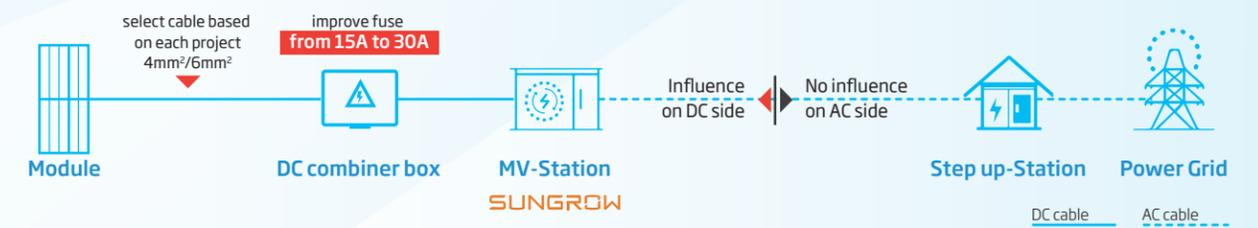
PV Module electrical diagram
