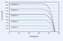
P-V CURVES OF PV MODULE(345W)
