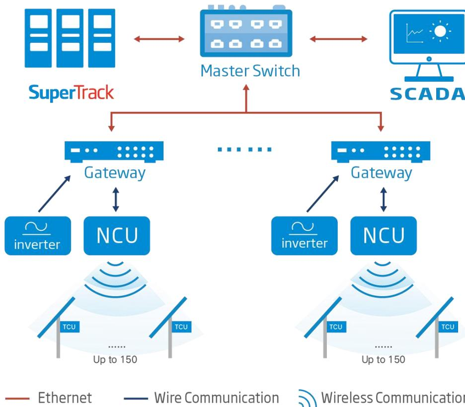
Trina smart tracking system consists tracker structures, tracker control unit (TCU), network control unit (NCU), SuperTrack platform and SCADA. Also, it can flexibly match with inverter and other equipment, thereby building integrated solutions to photovoltaic tracking system. (Figure 19)(Table 2)
