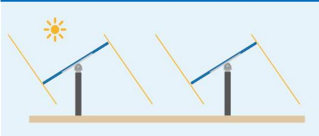
The conventional tracking algorithm consists of the astronomical algorithm and the backtracking algorithm. The scheme is characterized by simple control logic and strong engineering practicability, so
