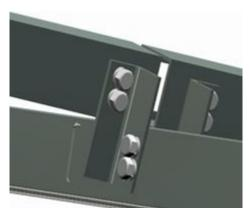
\*NOTE: For PV module landscape installation, the supporting rails need change as shown in below; (add two rails)
