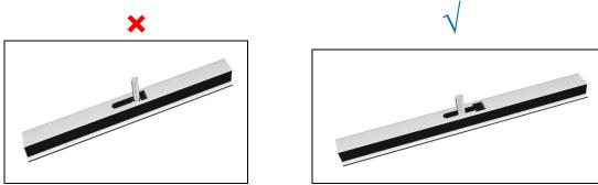
\*NOTE: Don't fix the hex nuts on head of the insert place. (As shown above). \*NOTE: Rack installation of connecting surface must sm $\sqrt{00}$  oth (As shown below).
