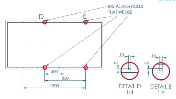
Figure 6 Mounting holes' schematic of the single module for the 2V installation method
