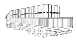
3.3.4 Only one-layer stacking is only allowed for small truck. Make sure that the package is fixed with packing straps securely to the shipping platform without movement.
