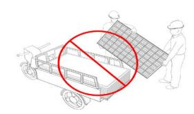
3.3.7 Do Not transport the module with rope as shown below:
