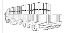
3.3.3 Transport: Do Not Stack more than two layers on truck;
