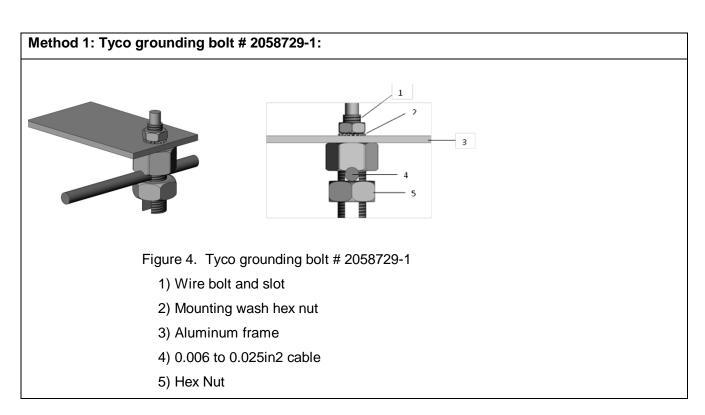
Tyco grounding hardware comes in a package that includes the grounding bolt, mounting and grounding hex nut.
