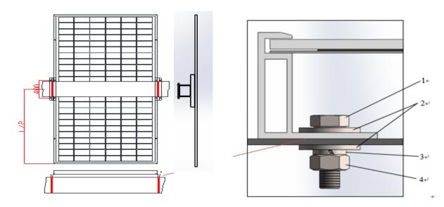
Fig 5. PV module installed with Single-axis Tracing System
