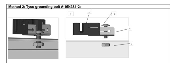
Figure 5. Tyco grounding bolt # 1954381-2 (NOT applicable for TRINAMOUNT module series)
