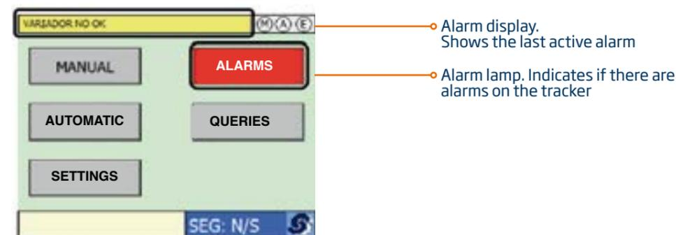
The last alarm that occurred in the tracker appears in the bar at the top of the screen. Keep in mind that the alarm that appears in the top bar is the last (but perhaps not the only) alarm. The alarm query screen can be accessed by clicking on the alarm display located at the top of the screen or on the flashing alarm lamp:
