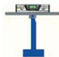
3. Move the tracker manually until it is completely horizontal (the digital level will read  $0^\circ \pm 0.5^\circ$ ).
