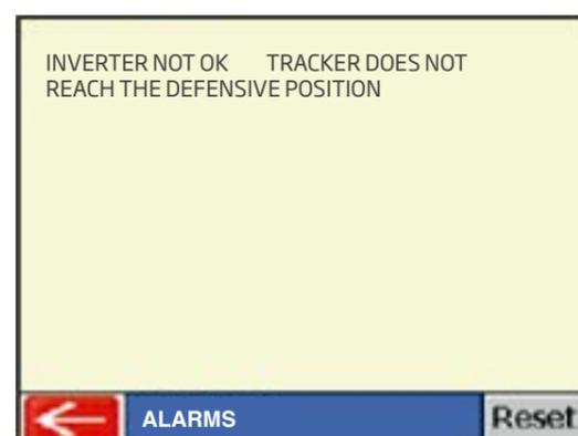
Press the "Reset" button to clear the alarms. It must be pressed in order to clear the alarms that require "reset". See section 3.3 of this manual for a detailed description of the tracker alarms.
