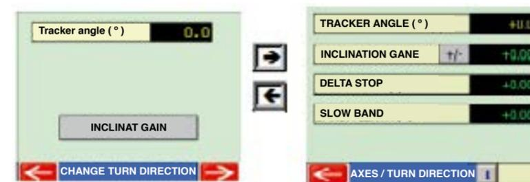
When the "CHANGE TURN DIRECTION" button is pressed, the direction of turning of the motor is reversed via software.
