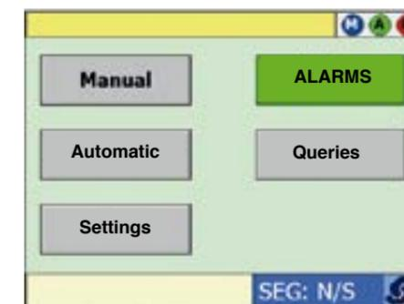
The tracker enters Manual Mode when the Manual button is pressed.
