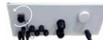
2. Unscrew the protective cap on the controller connector.
