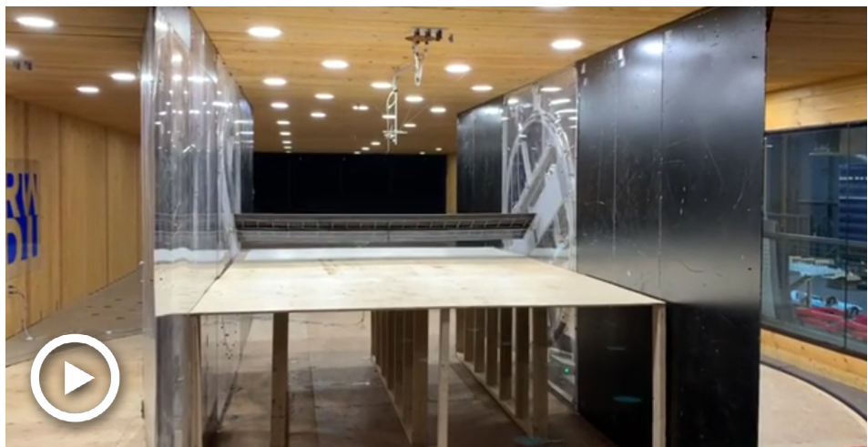
Image 29 - Video: 2D section model test. RWDI Lab
