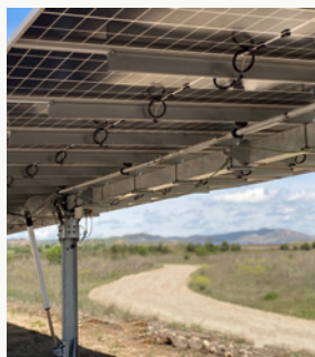
Image 7: Tracker testing under beta site conditions
