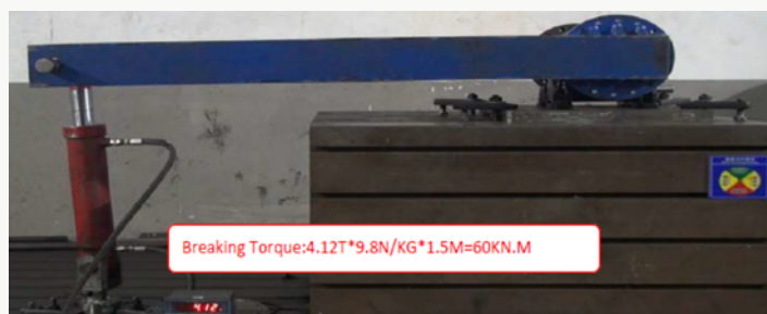
Image 16: Static maximum holding test
