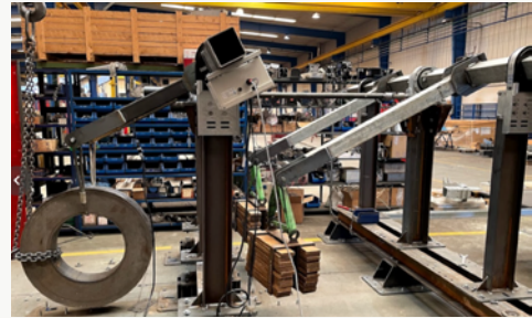
Image 17: Dynamic maximum load test
