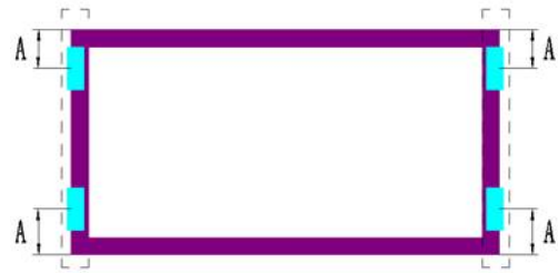
Use 4 clamps on the short side. Mounting rails run perpendicular to the long side frame.
