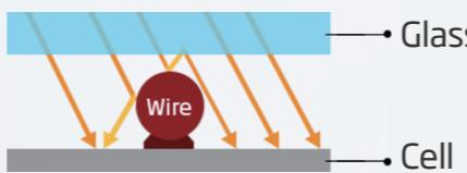
Multi-busbar technology, improving optical utilization rate with higher electricity performance
