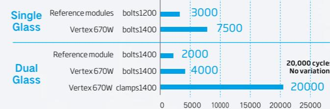
Extreme DML testing( $\pm 1500\text{Pa}$ ) ■ The number of cycles when a failure occurs
