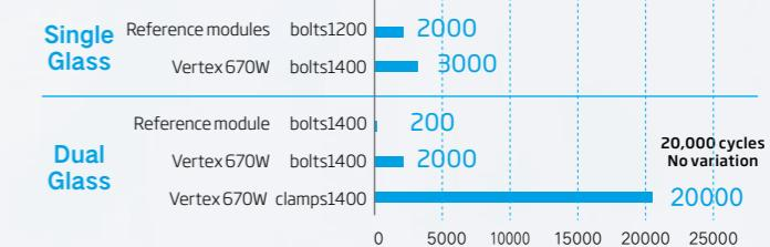
**Test results:** The appearance of the Vertex 670W module remained intact after 20,000 cycles based on the standard load of 1,000 Pa, the power degradation was 0.1%.
