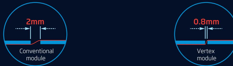
High density encapsulation technology, optimizing power output with good balance between reliability and efficiency, module efficiency increase 0.2~0.3%
