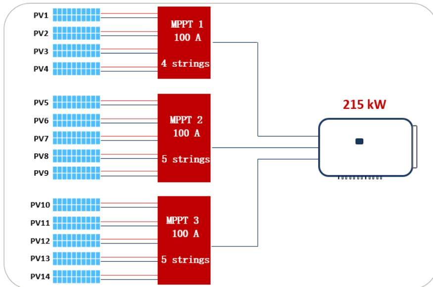
Figure 6 Inverter connection diagram of Circuit 3
