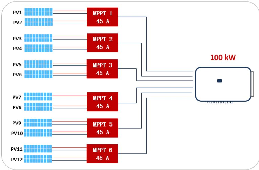
Figure 7 two strings connected into one MPPT
