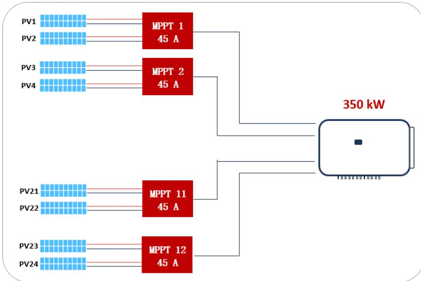
Figure 5 Inverter connection diagram of Circuit 2
