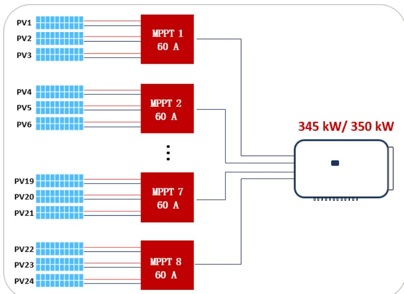
Figure 4 Inverter connection diagram of Circuit 1
