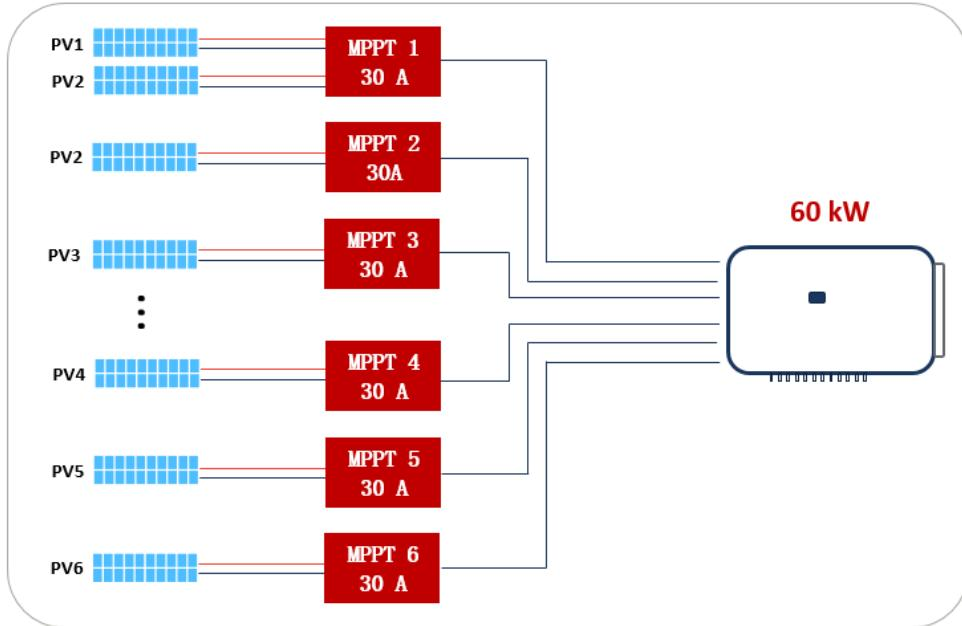
Figure 8 one string connected into one MPPT
