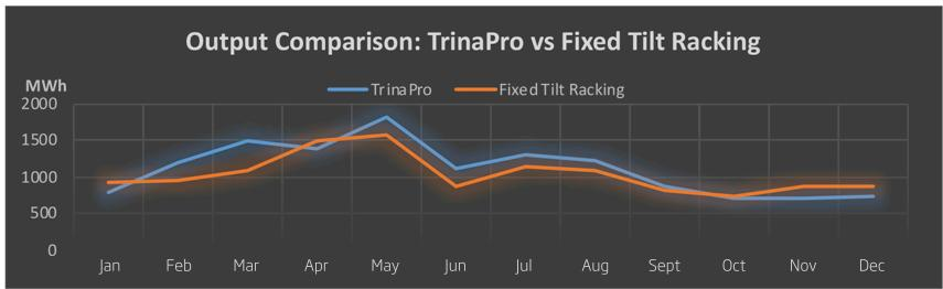
Affecting by the randomness of weather condition, TrinaPro's production is sometimes less than Fixed Tilt Racking's in Spring. Additionally, fixed racking system's production usually prevails during winter. However, TrinaPro's overall production still surpasses Fixed Tilt Racking's by 7.75% in the entire year.
